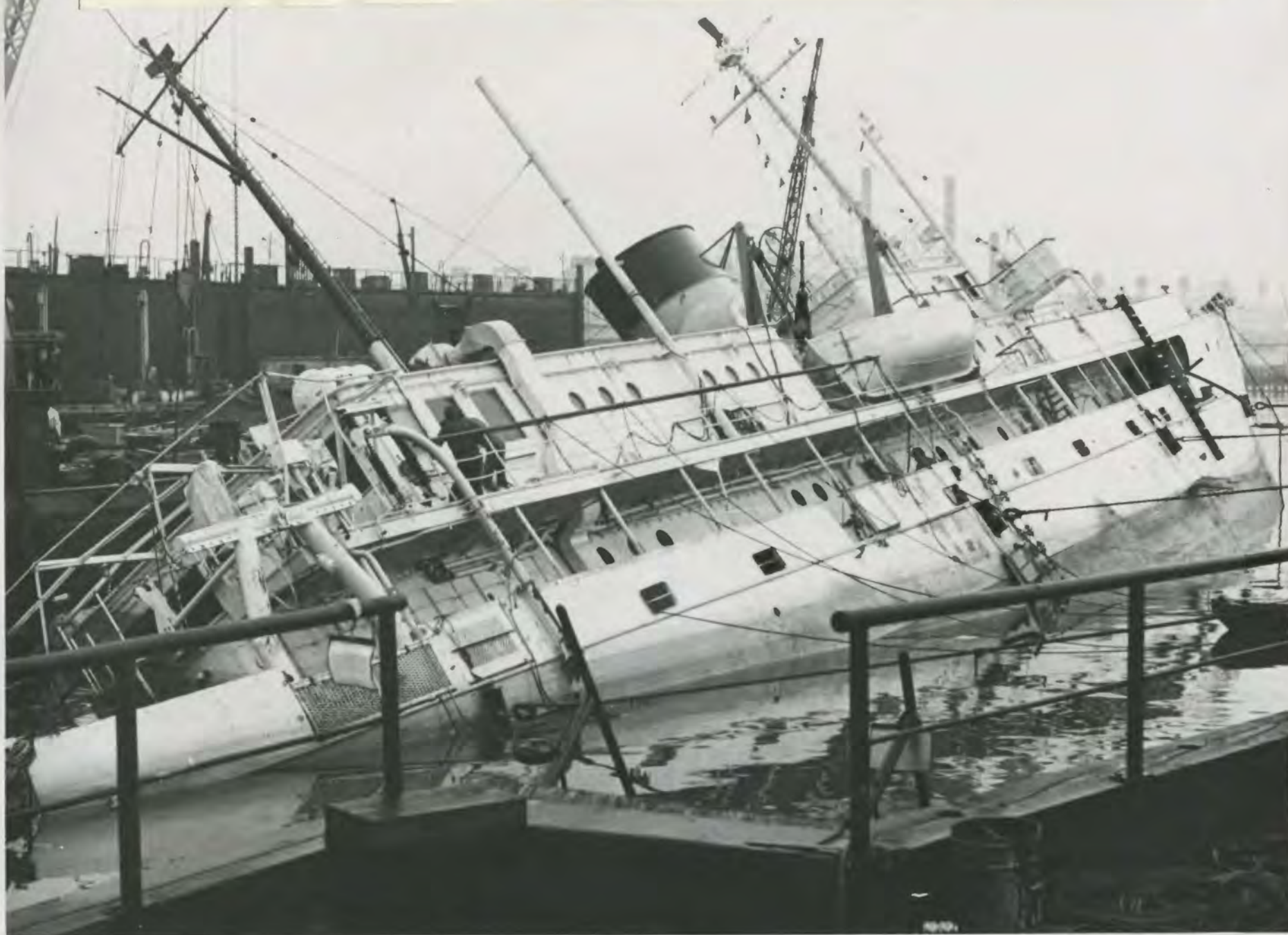
Figure 2- Starboard side of the R/V ANTON BRUUN as she lays capsized. The four restraining cables made fast to welded "pad eyes" on the vessel's hull are seen.
