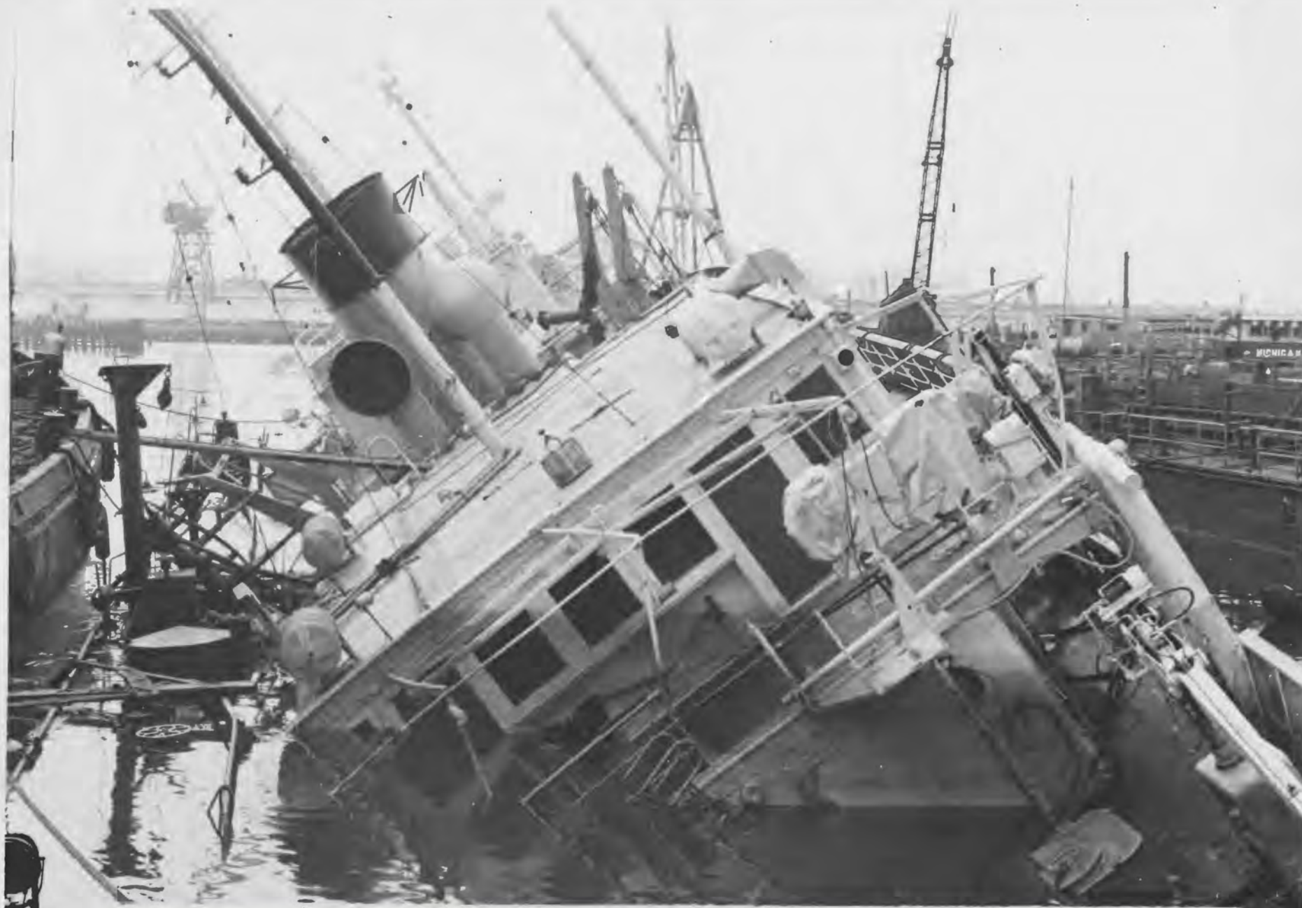
Figure 3- A stern view of the R/V ANTON BRUUN as she lays capsized. The high water mark can be seen on the vessel. Debris can be seen on the submerged port wing wall of the drydock. The salvage barge is at the extreme left of the photo. A ten inch pump can be seen spewing water to the right of the stack under the ventilator.
