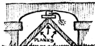
METHOD OF DESTROYING SMALL BRIDGES OR CULVERTS.
