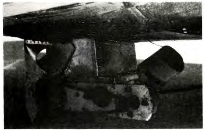
Homemade ejector on plane belly has distributed flies by the hundreds of millions over the huge Texas rangeland.
