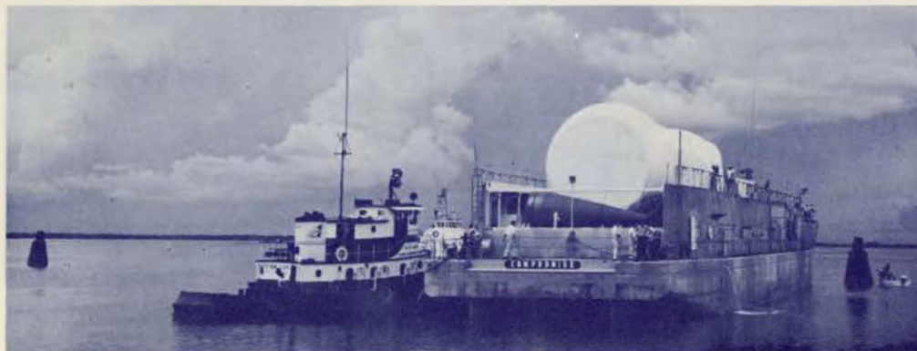
The Saturn SA-1 vehicle components aboard the barge Compromise during the trip to the Cape.
