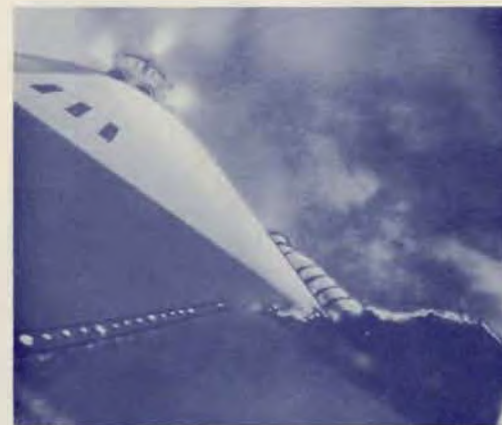
The S-IV stage blasts away from the S-I stage as separation is completed.
