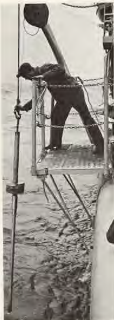
Samples of the ocean floor are retrieved with coring devices like these. The corer brings up a vertical, cylindrical specimen of the bottom sediment, from which the nature and stratification of the bottom may be ascertained.
