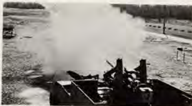
A 76mm test rig firing on a high velocity range operated by Development and Proof Services, Aberdeen Proving Ground, Maryland. The range is just one of the innumerable instrumented facilities available at APG for testing Army materiel.
