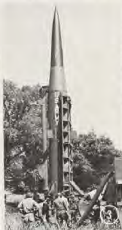
(1) At Hand Hill Firing Point, Fort Sill, Oklahoma, members of the 2nd Battalion, 44th Artillery, use a T-2 Theodolite to "lay-in" the Pershing missile. (2) A Sherman vehicle scales a barrier on the Munson Test Course at APG. (3) Crew members watch as Pershing missile is raised on an erector launcher vehicle at Fort Sill, Oklahoma. (4) A Lance Missile System vehicle completes a swimming test at APG, Maryland. (5) Pershing moves horizontally, too. Here, crew members perform inspection before moving out of training area to firing area. In front is the XM-474 warhead vehicle and behind is the Pershing erector launcher vehicle. Fort Sill, Oklahoma. (6) At APG's Munson Test Course a 2,500-gallon tanker is put through a durability test. Munson is one of APG's automotive facilities for testing of Army combat vehicles and other wheeled and tracked equipment. (7) The XM410E1, a new 2½ ton cargo vehicle
