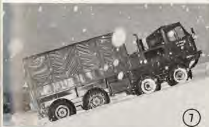
with eight wheels and a sophisticated system of suspension and power transfer, attacks the snow covered slopes of the Arctic Test Center's incline test facility. (8) Soldier-technicians bake up a batch of bread rolls in an experimental Continuous Bakery System at the General Equipment Test Activity, Fort Lee, Virginia. This system was developed to satisfy military requirements in supplying fresh bread to combat troops in the field. The system is ultimately intended to replace the Army's Standard Mobile Field Bakery presently in use. (9) The Honest John Artillery Rocket on a test launch from White Sands Missile Range, New Mexico. (10) Besides its bout with the snow (photo 7), the new "eight by" must also take on the mud. This mud test was conducted by the Armor Board, Fort Knox, Kentucky.
