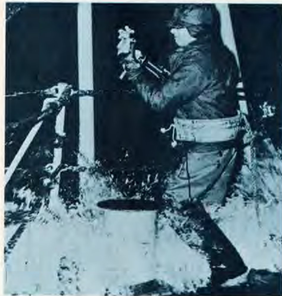
A seaman prepares to make Nansen cast in rough seas at night. The Nansen bottle is a traditional oceanographic instrument used to retrieve samples of sea water. It is equipped with a rotary valve at each end so that when it is rotated at depth the valves close and lock shut, entrapping a water sample and setting reversing thermometers. The bottle is named for its designer, Fridtjof Nansen.
